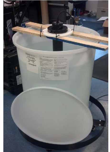
Figure 1. Current Sensor In-Water Testing
