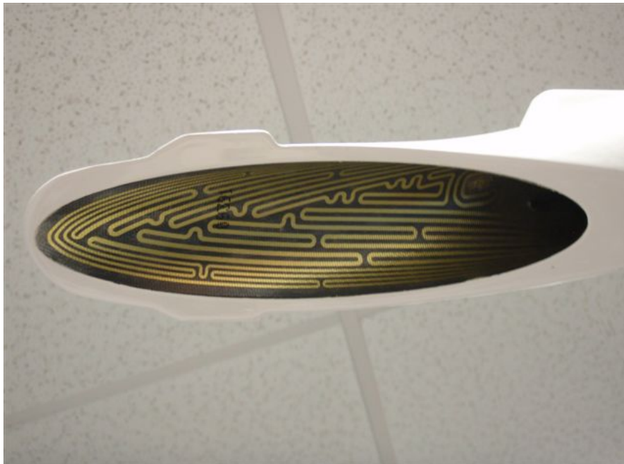
Figure 8. Heaters on the underside of the hood.
