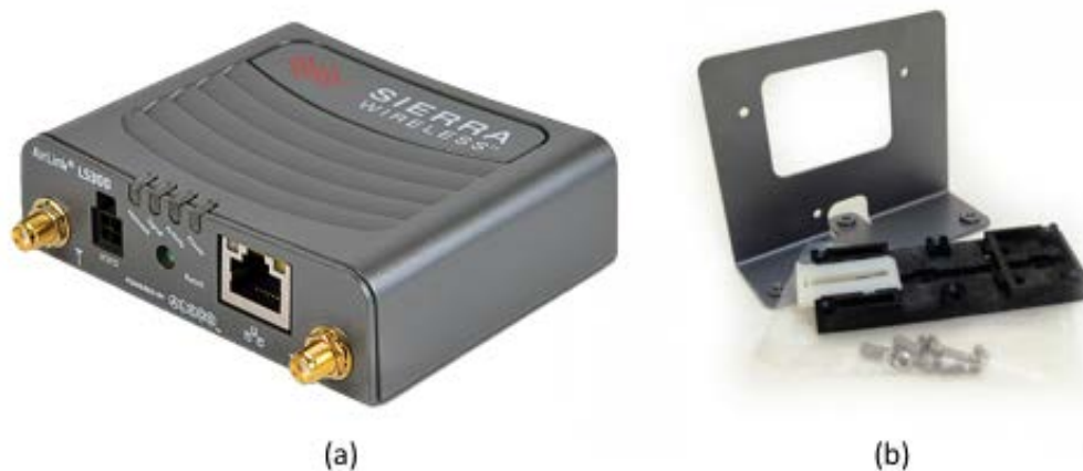
Figure 32. IP Modem - LS300 and mounting bracket
