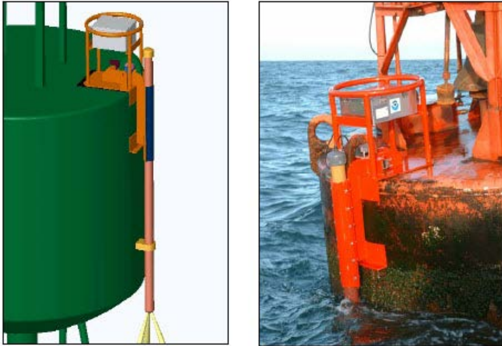
Figure 3. Diagram (l) and picture (r) showing the ATON ADCP system's Clamparatus that is used for attaching the downward-looking current profiler.
