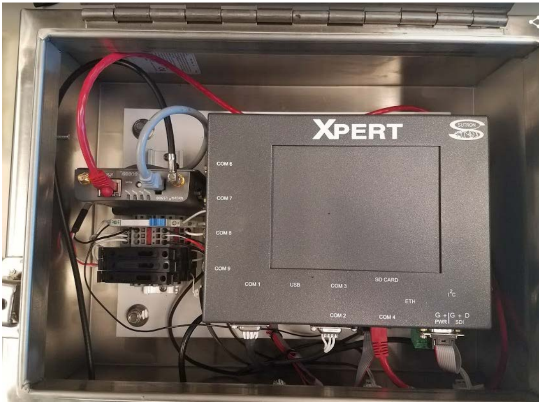
Figure 14. iATON electronics enclosure configuration and wiring EXAMPLE
