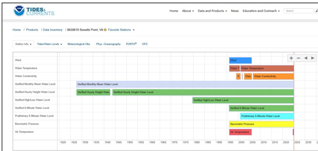
Figure: Data inventory for 8638610 Sewells Point, VA. The 6-minute height and high water analysis uses Verified 6-Minute Water Level and the Verified High/Low Water Level. The hourly height analysis uses the Verified Hourly Height Water Level.
