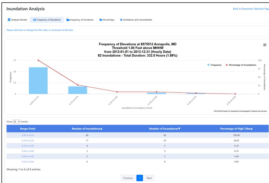
Figure: Frequency of Elevations plot after the range was adjusted from 0.05 feet to 0.1 feet.
