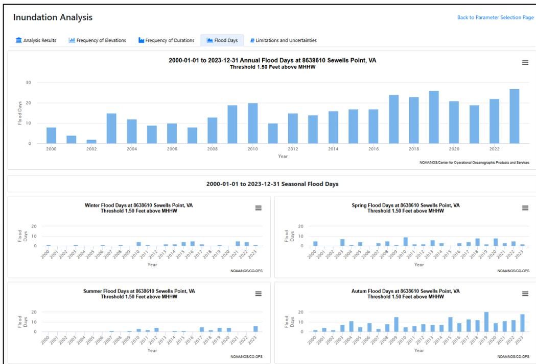
Figure: Flood Day plot for 8638610 Sewell's Point, VA using a threshold of 1.50 feet above MHHW. Since this threshold is lower than the NOS threshold of 1.75 feet above MHHW, the number of flood days is higher than the “official” NOS flood day count for this station.
