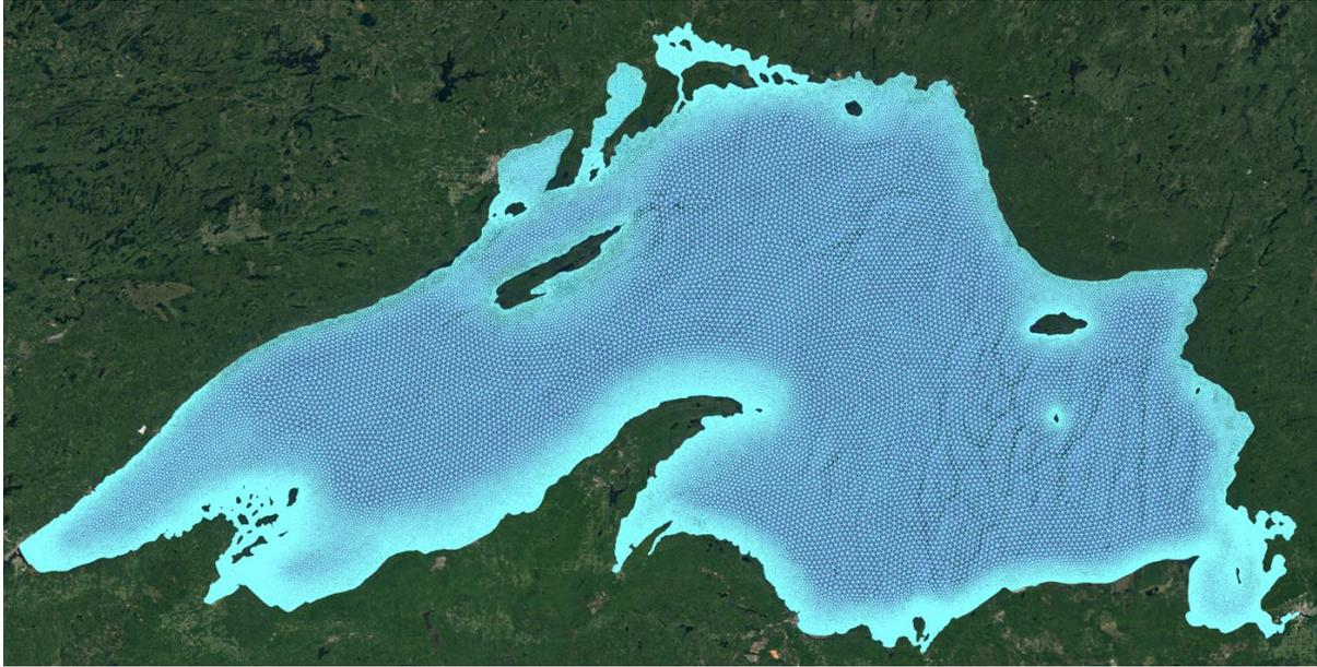
Figure 2. Map depicting the FVCOM grid domain for LSOFS. The horizontal resolution ranges from around 200 m (0.12 mi) near the shore to approximately 2.5 km (1.6 mi) offshore with 21 vertical sigma levels.
