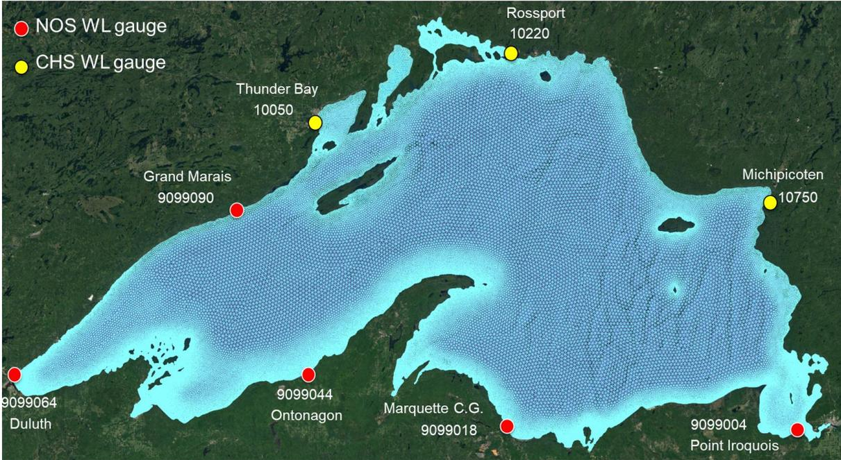
Figure 7. Locations of NOS and CHS water-level gauges used to evaluate LSOFS water level hindcasts.
