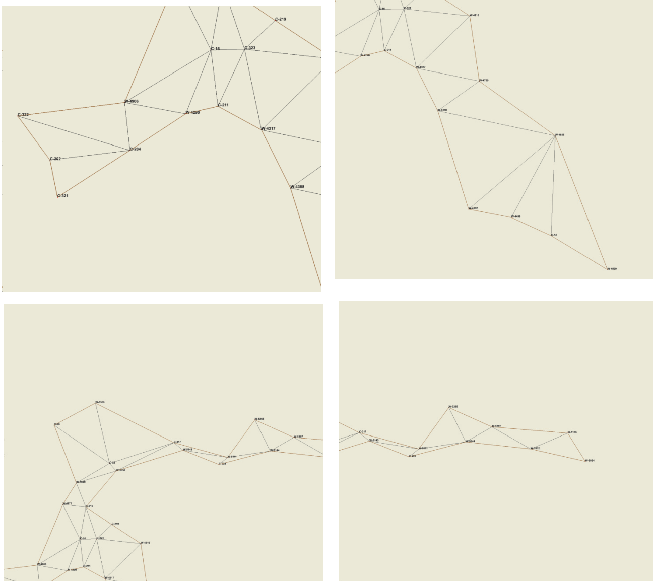
Figure 2.20. Unstructured Salinity and Temperature Initial Condition Grid, with the appropriate water level and CT stations assigned. Note it was necessary to assign synthetic CTD profiles to each station based on CT and CTD data.
