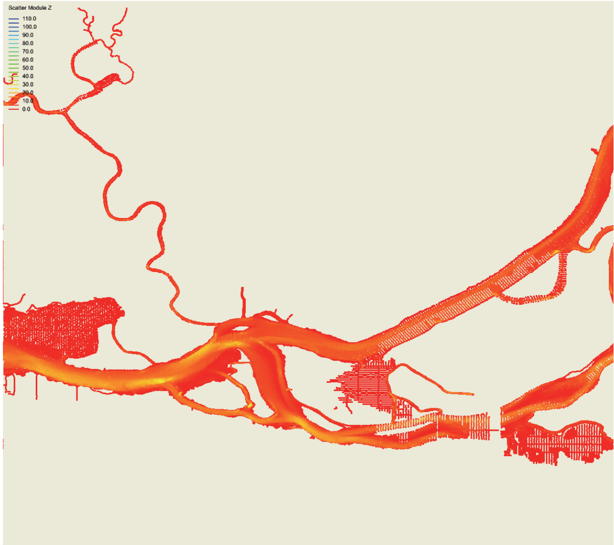
Figure 2.9. San Francisco Bay Delta Hydrographic Survey Data in meters.
