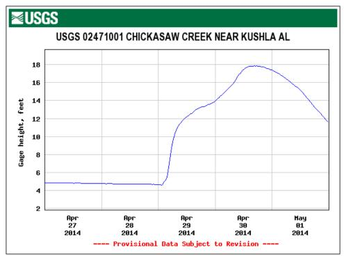
**Figure 3**. USGS river gage at Chickasaw Creek, AL, about 3 mi upstream of the CO-OPS Chickasaw Creek station (8737138), measured a sudden increase in river levels. At the time that this station's river levels rose (~18:30 GMT), the water levels at 8737138 were only about 2.0 to 2.5 ft above MLLW.
